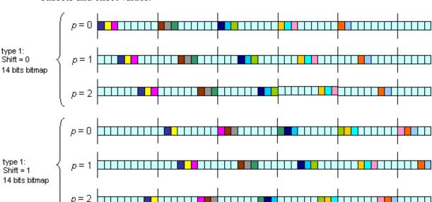
inside a selected subset. The figure shows all the bits in Bitmap set to '1' for different subsets and offset values.
